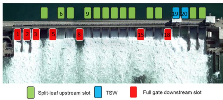
If lower flows are forecasted and meet all hydrologic criteria below, crews will open double-leaf gates 1 and 2 in the downstream slot to 4 stops (~7 kcfs spill) each on April 10 as early as possible during daylight hours and spill will be distributed according to patterns in **Table MCN-8-ALT**. From 0001 hours until gates 1 and 2 are opened, spill will be at the FOP target using patterns in **Table MCN-8**:
