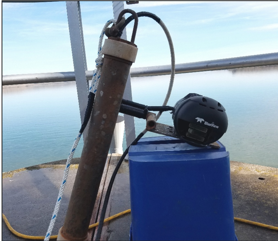
Figure 2.4. Imaging Sonar Attached to Trolley and Prior to Deployment into the Trolley Pipe
