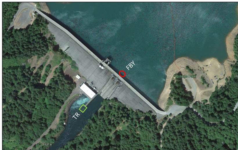
Figure 2-1. Radio telemetry detection locations to assess survival and behavior of juvenile Chinook salmon at Green Peter. The red circle depicts the forebay antenna (FBY), and the green square depicts the tailrace antenna (TR).
