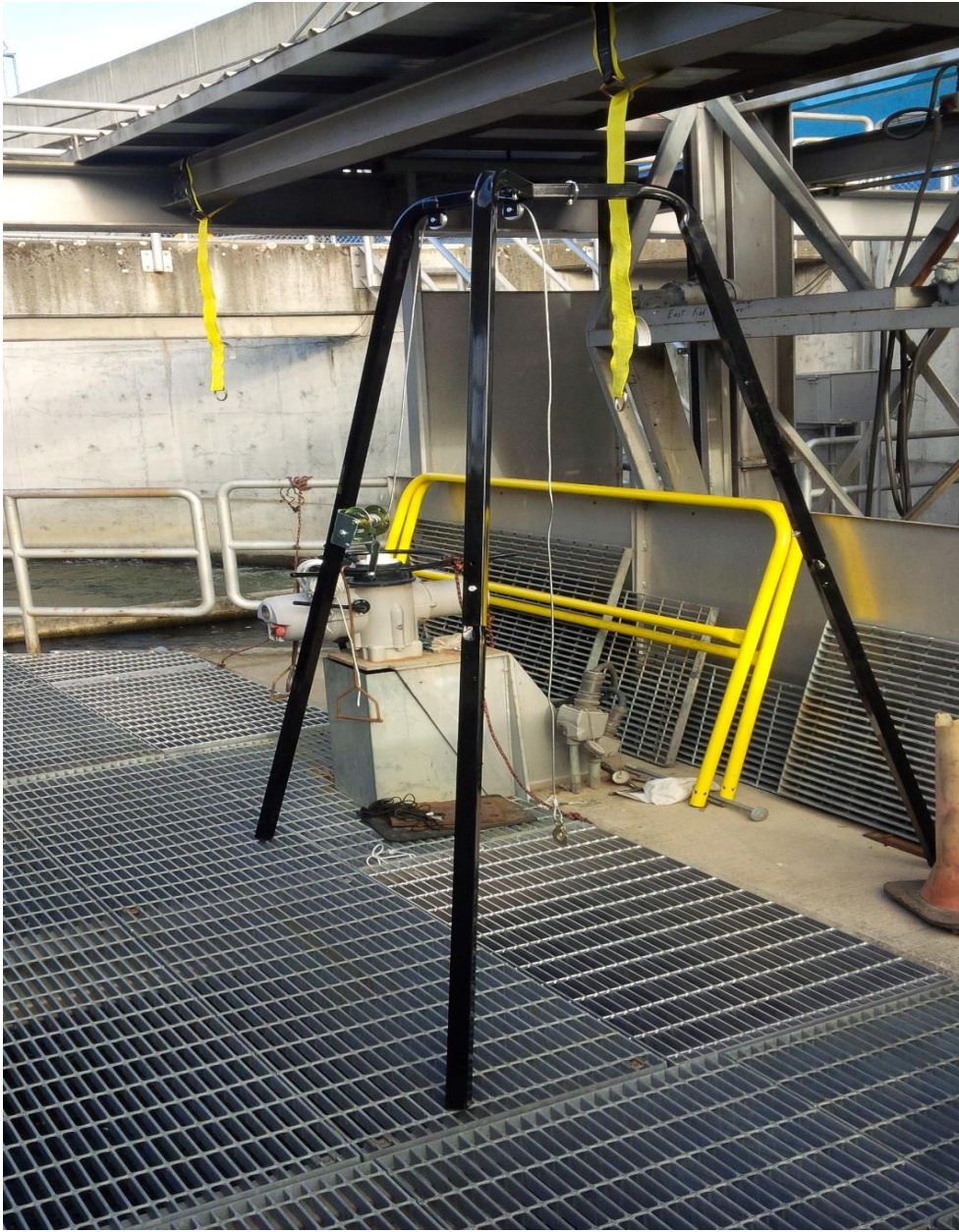
Hoist purchased to assist tribal lamprey trap removal at east count station.
