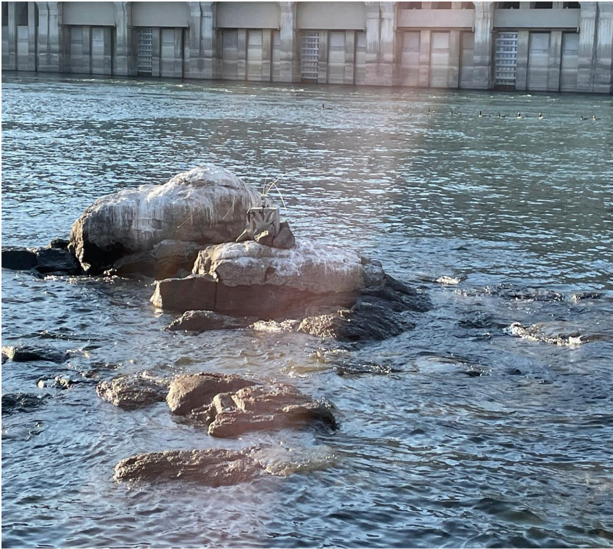
Gadfly noisemaker and "long legs" bird deterrents able to reduce cormorants on shoreline. Had to be relocated
