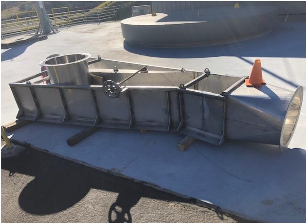
New PUD bypass switch gate ready for install.
