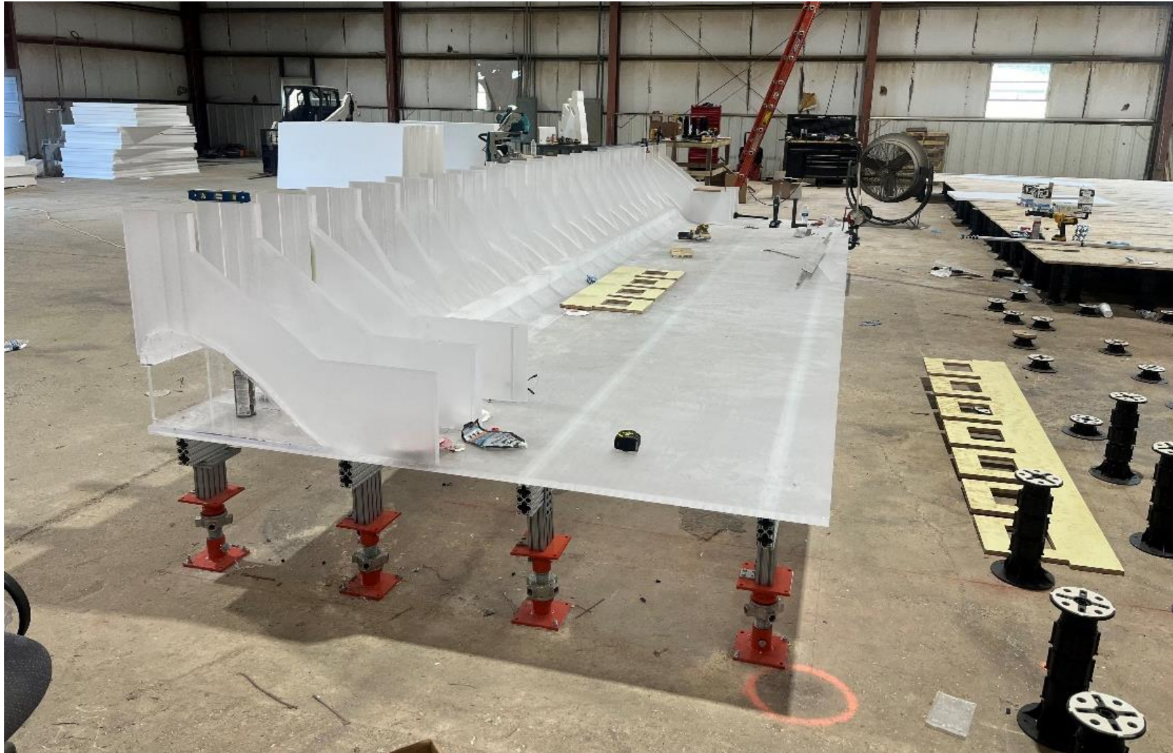
Spillway in place at model
