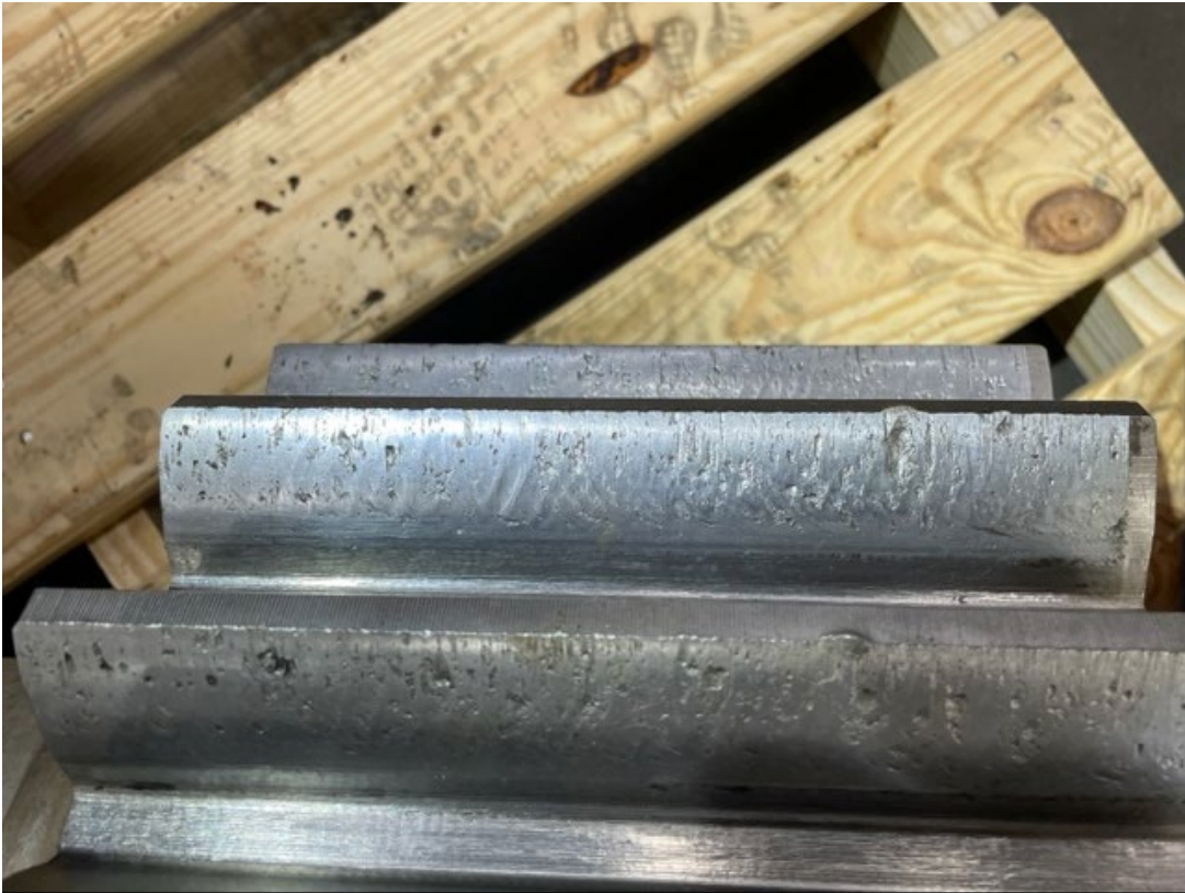
Pitting on south pinion gear
