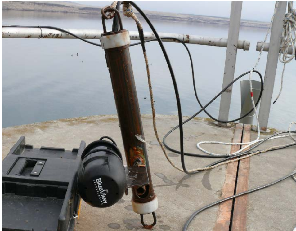
Figure 2.6. BlueView Imaging Sonar Attached to Trolley and Ready for Deployment
