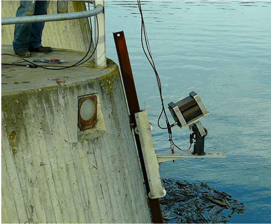
Figure 2.3. DIDSON Mounted to Rotator and Trolley Prior to Being Deployed at Unit 5/6 Main Pier Nose
