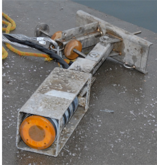
Figure 2.1. Transducer Installed in an Adjustable Mount and Prepared for Installation
