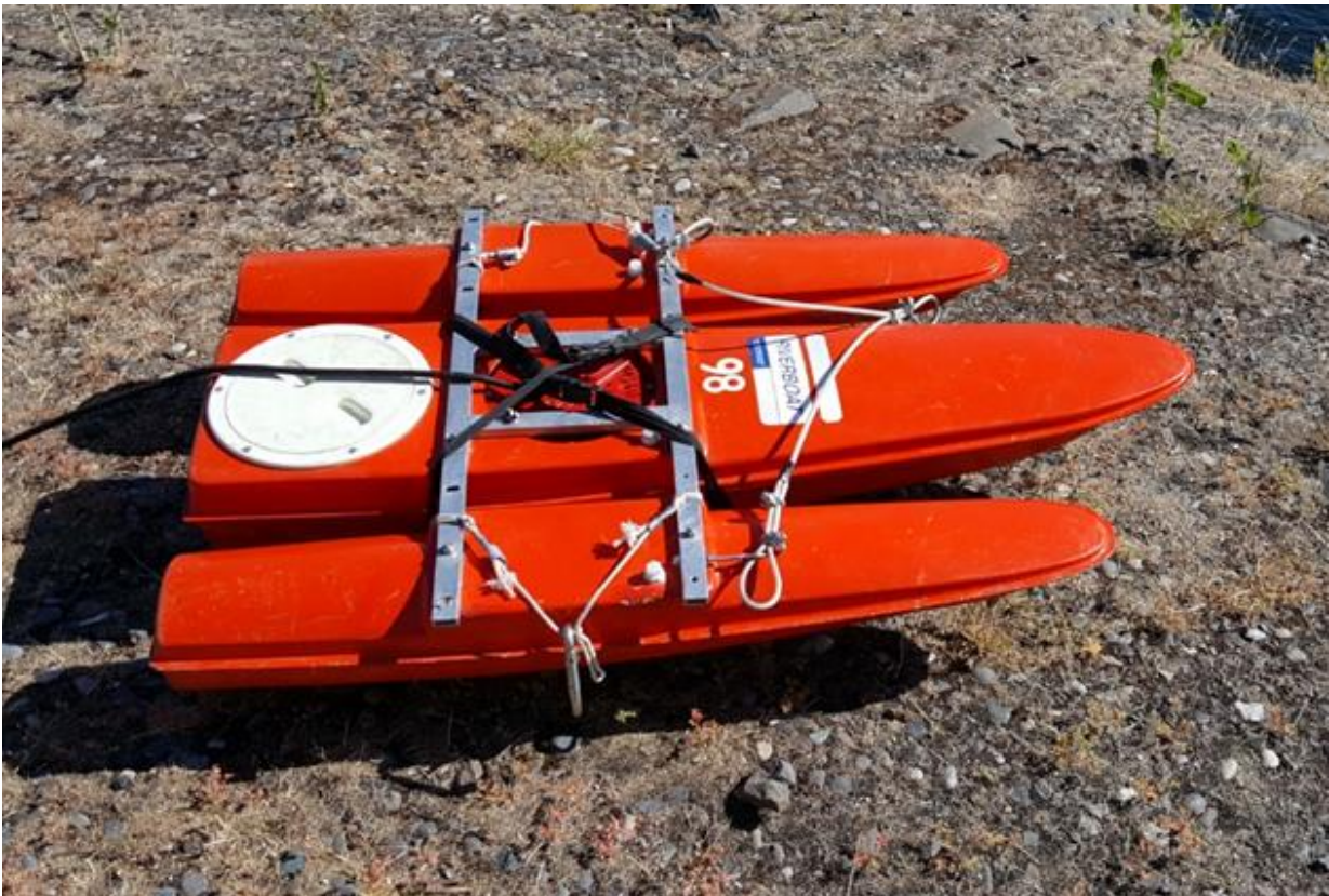
Figure 12 Photograph Showing Acoustic Doppler Current Profiler Unit Mounted on a Trimaran
