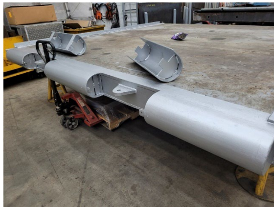
Figure 2: Picture of the rounded top on the newly modified SE-1 weir. The rounded top will make it easier for lamprey to enter the ladder. Once deployed the detached rounded sections (shown sitting on top of the weir) will mount over the lifting brackets.
