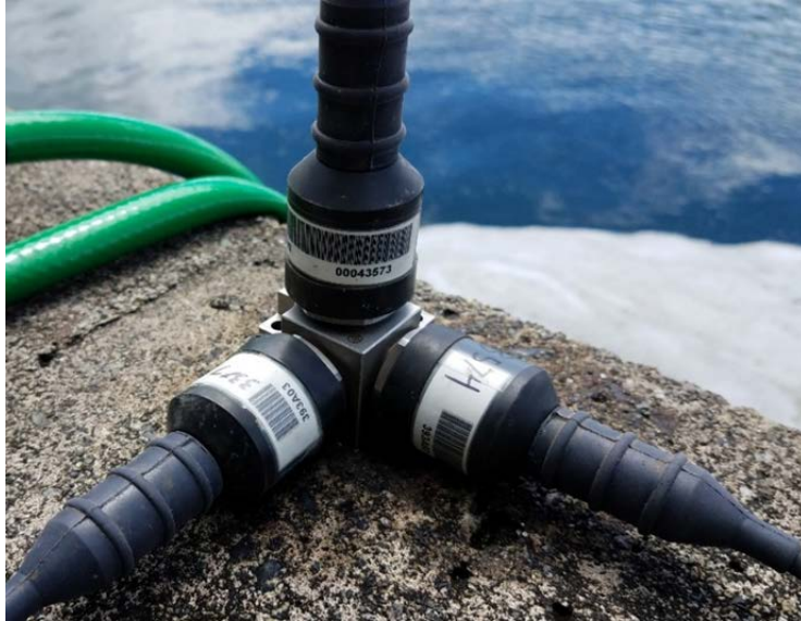
Figure 2.4. Photograph PCB Piezotronics Model 393A03 Single-Axis Accelerometer. Accelerometers were installed in a tri-axial array at each of the measurement sites.
