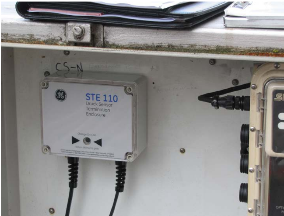
Figure B1.6.4 A Second Type Level Transducer, Preferred by the Corps because it has Moisture Preventative with Indication
