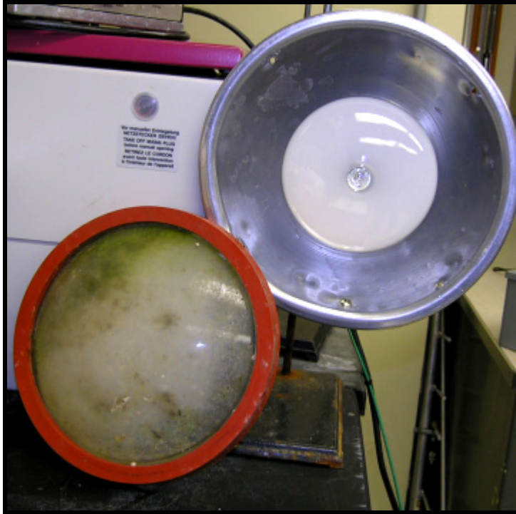
Figure 2.12. Water-scaled orifice tube lens cover (left); mercury vapor bulb with heat shield (right)
