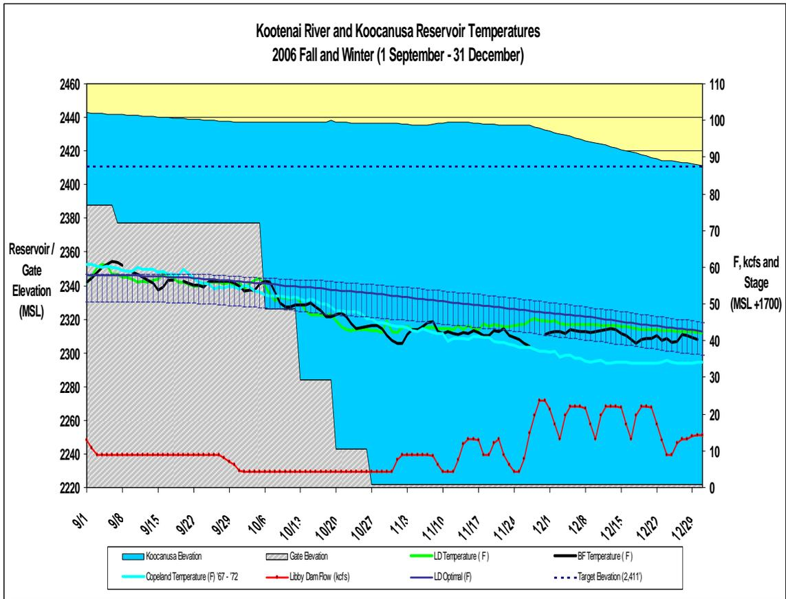
Figure 3. 2006 Libby Dam selective withdrawal gate removal, reservoir elevation, and Kootenai River flow and temperature data. The Copeland gage is downstream of Bonners Ferry, Idaho.
